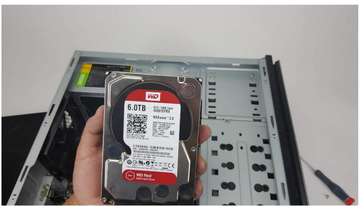
Step 7. Take note of the make and model of the hard drive, and the type of connector.
